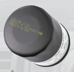
Most AMSOIL Oil Filters feature a reference arrow to aid in proper installation. Once the filter is finger tight, it is easy to gauge the additional .75 to 1.25 turns required to ensure a good fit. Over-tightening can lead to leakage.
